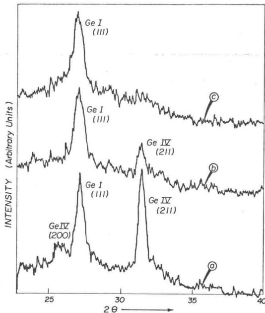
Fig. 3. Portions of X-ray diffraction traces made using  $\text{CuK}\alpha$  radiation illustrating the transformation from Ge IV to a non-crystalline product. Note that the Ge I peak does not increase in intensity, whereas the broad non-crystalline background does. (a) immediately after run, (b) after  $\approx 48$  h at ambient conditions, (c) after  $\approx 150$  h at ambient conditions.
